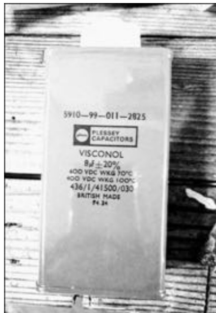
Photo 6 – Possible PCB Containing Capacitor
