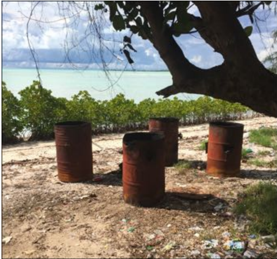
Photo 16 – Corroded Drums Currently Used for Clinical Waste Incineration
