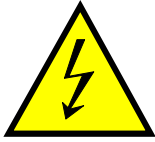
Figure 4 Marking of high voltage equipment
