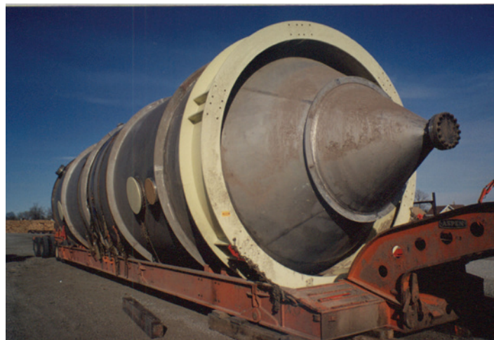
Figure 13 2205 batch digester for a Canadian pulp and paper mill
